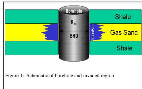
Figure 1: Schematic of borehole and invaded region
