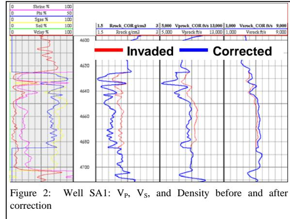
Figure 2: Well SA1:  $V_p$ ,  $V_s$ , and Density before and after correction
